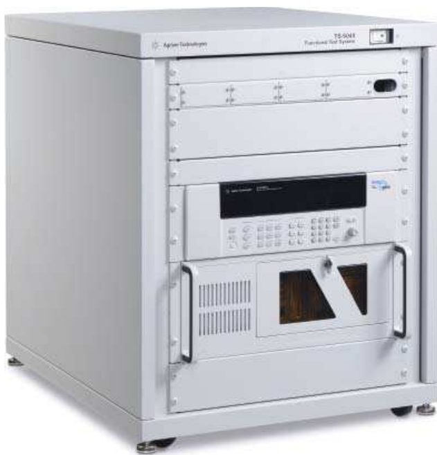
Figure 1. TS-5040 entry functional system
