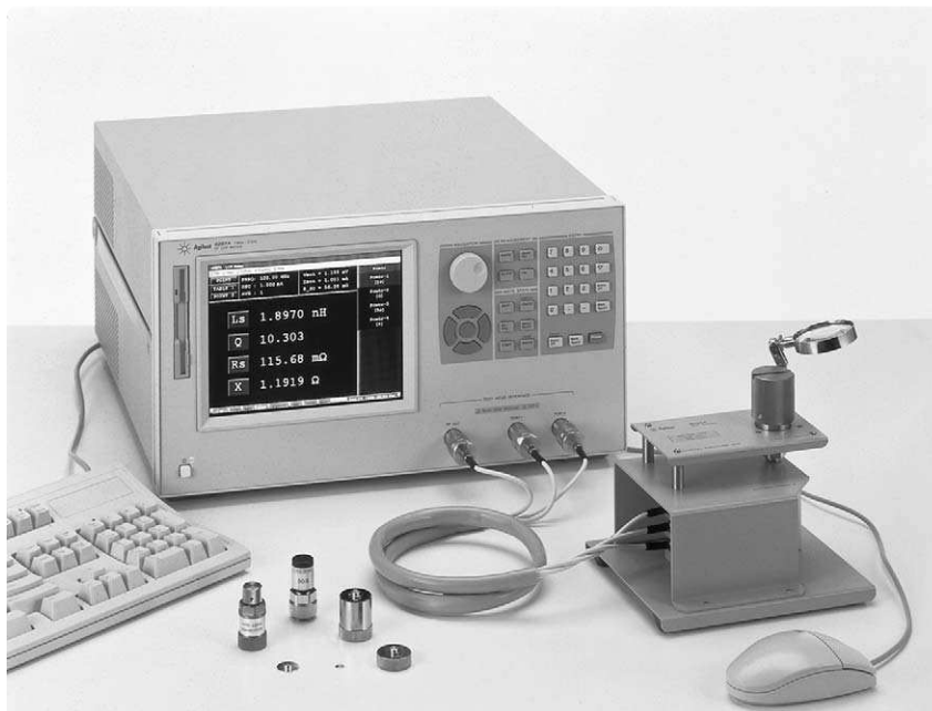
Figure 9. Total measurement solution example (with 16196A)
