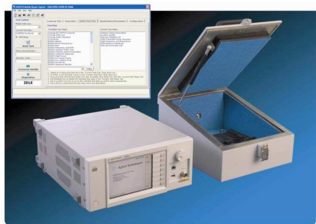
Figure 1. GS-8210 test system with N9360A, shield box, and test software
