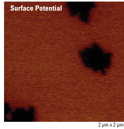
AFM studies of fluorinated alkanes adsorbed on silica using KFM. The aggregates exhibit a different surface potential with respect to the substrate.
