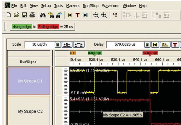
Figure 9. Use markers to measure the time between the rising edge and falling edge on a signal of interest
