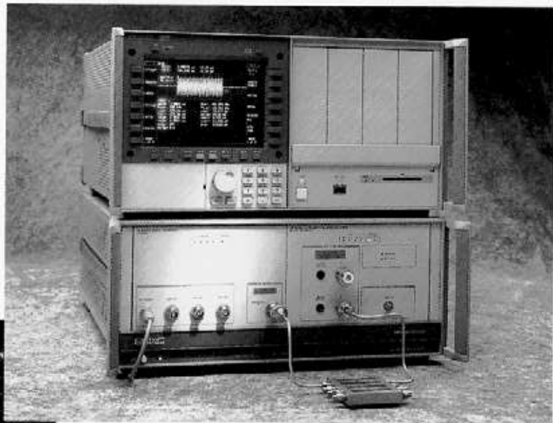
Excellent pulse fidelity makes the HP 70340A an ideal pulsed component and EW receiver stimulus.
