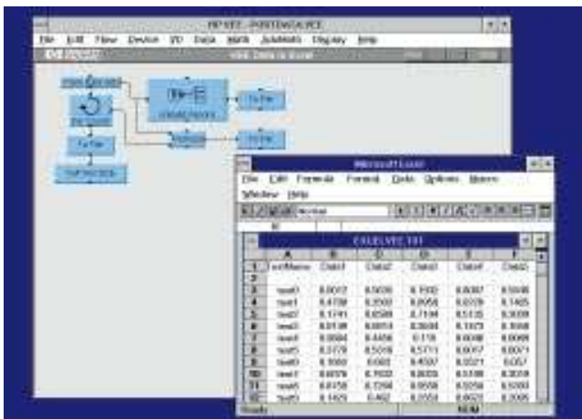
This HP VEE program uses DDE to send test data to a Microsoft Excel spreadsheet automatically.
