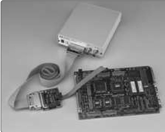
Figure 1: Standalone Agilent Technologies Emulation Probe
