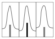
With just a glance at the gain bars, you can tell if your tuner output power meets specification during reference track (relative) measurements.
