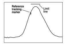
A combination of reference tracking and limit lines let you easily make peak-to-carrier measurements such as peak-to-video, peak-to-audio, and peak-to-color.
