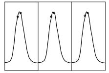
The 8730A displays up to four different sweep segments simultaneously so you can easily perform multichannel alignment.
