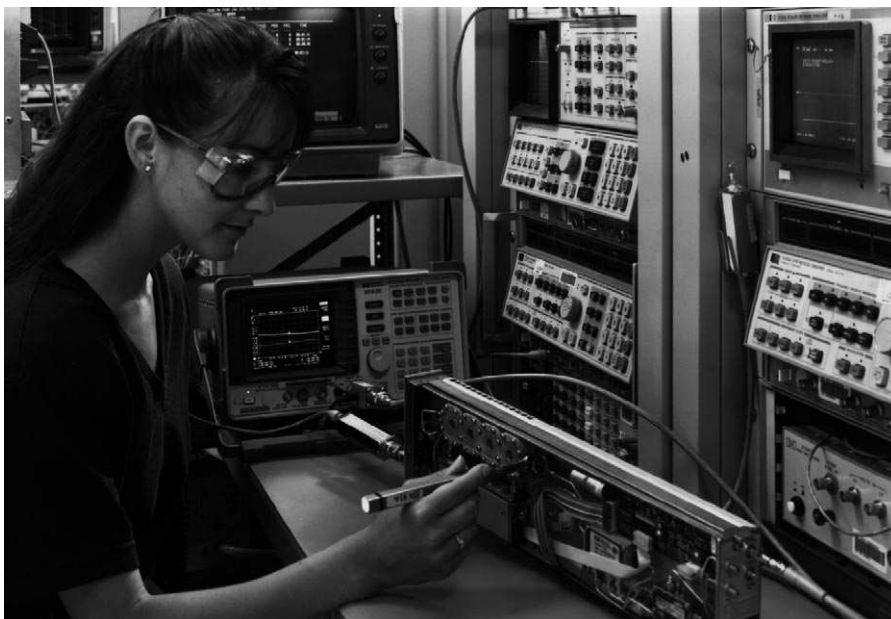
A narrowband amplifier is measured in a 100 kHz bandwidth.
