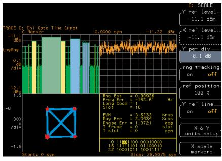
Examine the composite code-domain power display (upper left) while simultaneously viewing composite power versus time (upper right), symbol constellation (lower left), and modulation metrics (lower right).
