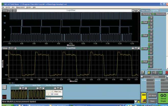
Figure 3. Logic View allows you to visualize and analyze up to 16 digital signals and 4 analog signals simultaneously for maximum insight.
