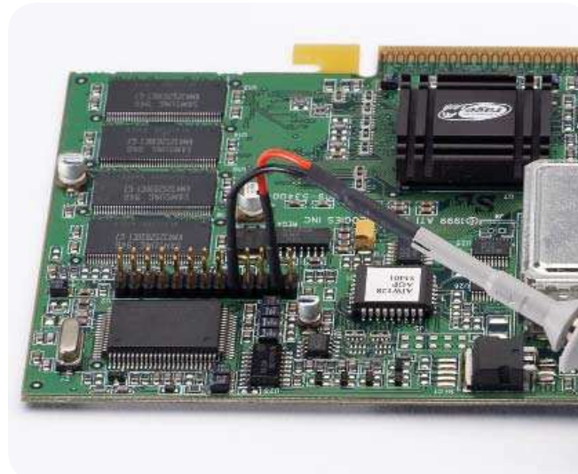
Figure 7. The dual lead adapter allows you to easily connect the N2870A Series probe to a popular 0.1" pin header with 0.025" square pins. This dual lead adapter has no shorting hazards since all external metal surfaces are insulated.
