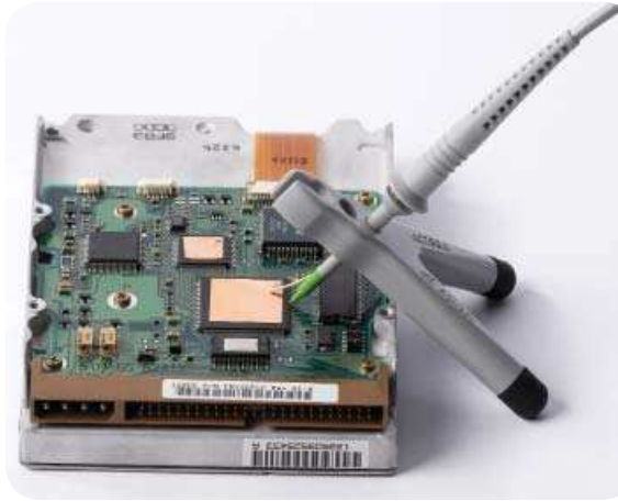
Figure 8. An IC cap adapter and ground blade with optional N2786A two-leg probe positioner offers an ideal hands-free solution for short circuit-proof probing of a fine-pitch IC. The N2877A deluxe accessory kit and N2878A fine-pitch accessory kit contain one N2786A two-leg probe positioner.
