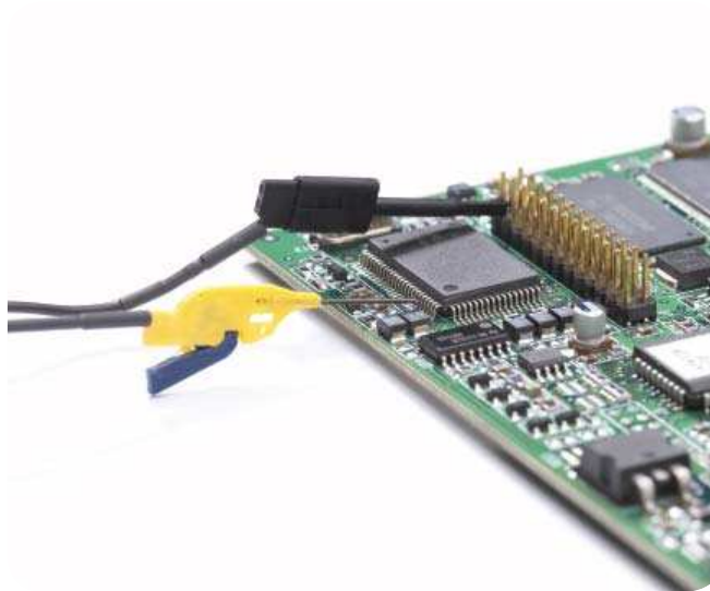
Figure 6. With today's miniature IC- and component-packaging techniques, probing can be a considerable challenge. Use 0.5 mm QFP IC clips with TQFP/PQFP packages with 0.5 mm lead pitch or greater, or use pico-hook clips made for connections over components or wires with leads up to 0.04" diameter or smaller.
