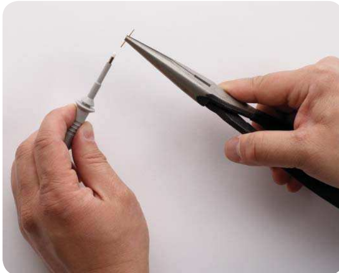
Figure 2. Sharp probe tip makes it easy to probe today's fine pitched components.
