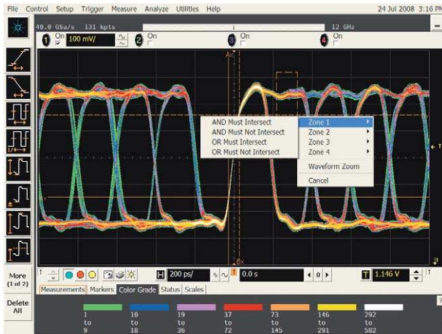
Figure 7. The InfiniiScan zone qualify finder is used to isolate single-bit pulses. Only the waveforms that pass the must-not-intersect (upper left) and must-intersect (lower right) graphical zones are displayed.
