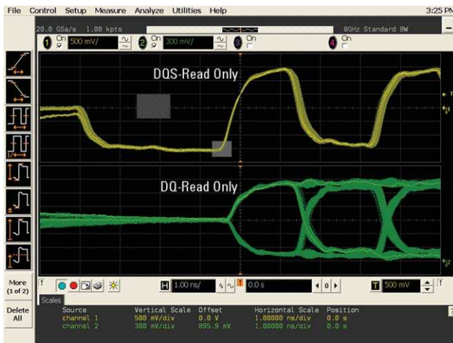
Figure 9. Notice how zone qualify is able to easily isolate the exact signal you need. This is very useful for many applications, including separating reads and writes for memory signals.
