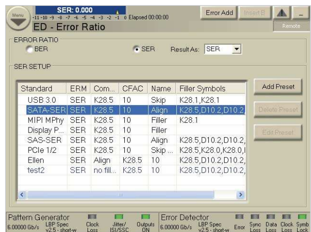
Figure 29. SER analysis option enables receiver tolerance testing of devices using retimed, coded loopback.
