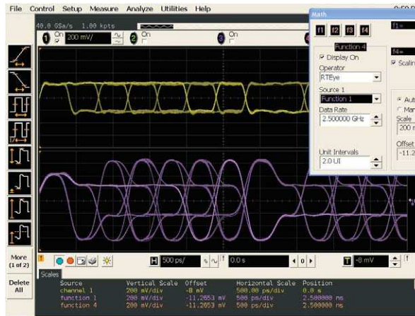
Figure 4. The signal on channel 1 went through linear feed-forward equalization and is displayed in function 1.
