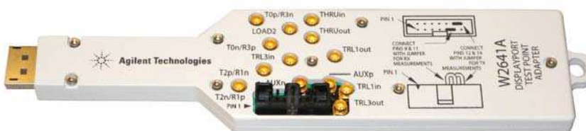
Figure 8: W2641A DisplayPort test point access adaptor.
