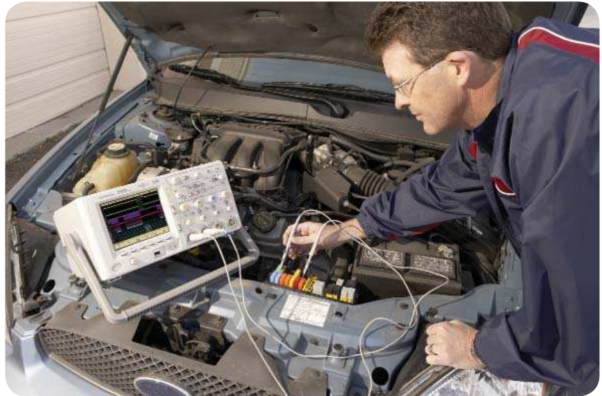
Figure 12: Making remote FlexRay measurements with Agilent’s battery option for InfiniiVision Series scopes
