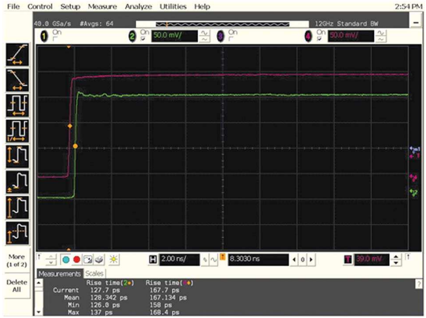
Figure 5 Time domain single-ended probe response, purple = input of the probe, green = probe output, using Agilent 1169A InfiniiMax probe and DS081304B 13 GHz oscilloscope
