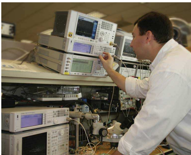
Express MXG analog signal generators cover a wide range of applications including local oscillator (LO) and clock substitution; continuous wave (CW) interferers; power calibration; antenna testing; and analog communication systems that use AM, FM or phase modulation.
