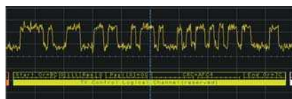
MIPI DigRF v4 decode embedded in waveform area
