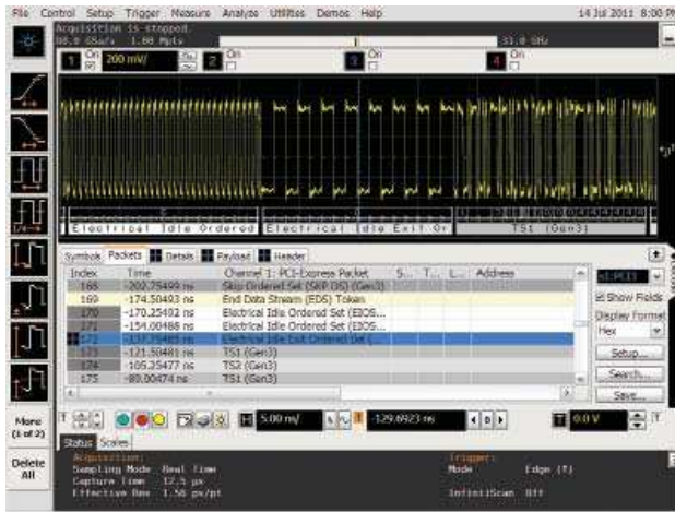
Figure 3: The packet-level decode below the correlated portion of the PCI Express signal
