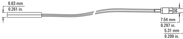
Figure 3.6. E5394A and E5396A soft touch probe dimensions
