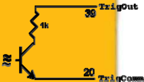
Trigger Output Optical Isolator NPN circuit.
