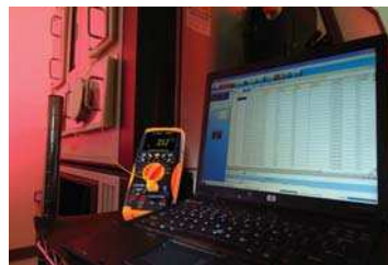
Figure 1: Automate recording of measurements with bundled GUI data-logging software.
