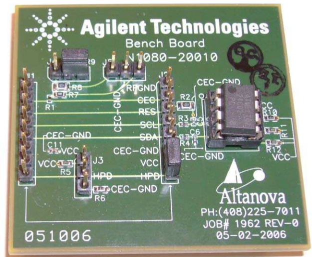
Figure 5b. The N1080A H06 test point adapter
