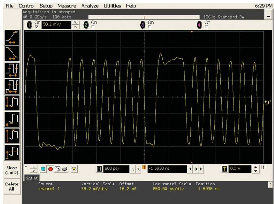
USB 3.0 supports the data rate of 5.0 GT/s as shown above (~3.5 dB de-emphasis)
