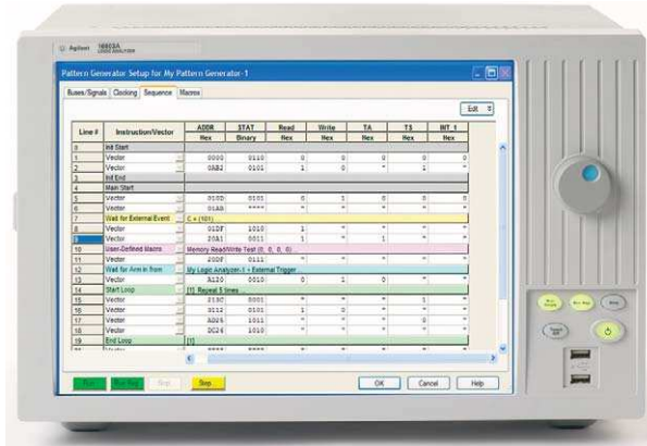
Figure 3. Models with a built-in pattern generator give you more measurement flexibility.
