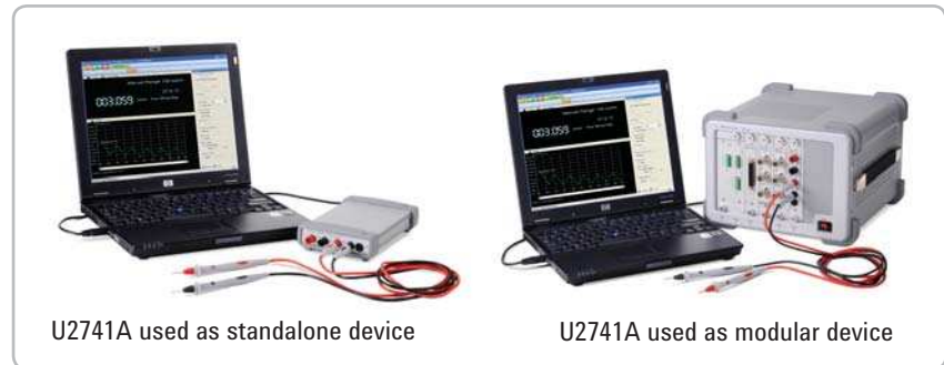
Figure 1. The U2741A DMM showing dual-play capability
