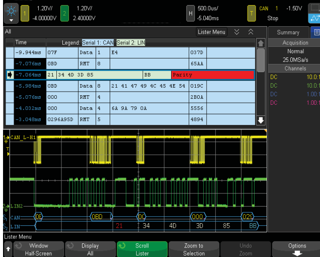
Figure 3: An interleaved “Lister” makes it easier to time-correlate activity between two decoded serial buses.
