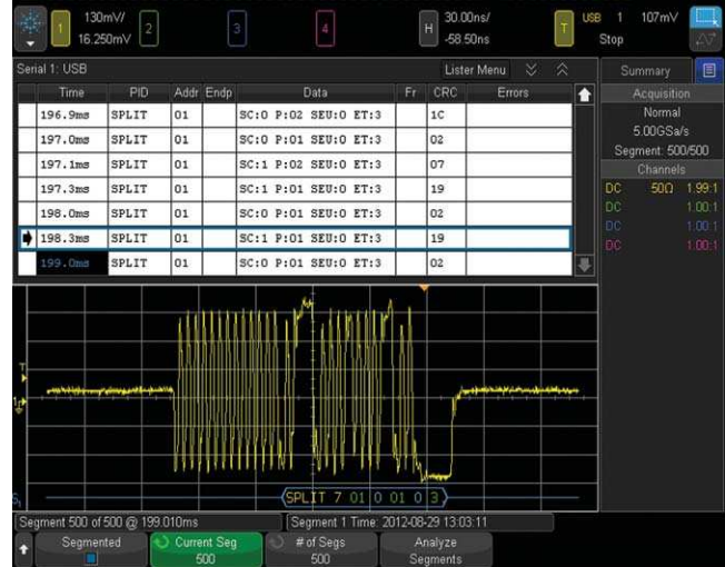
Figure 4: Segmented memory acquisition selectively captures more packets/bytes of serial bus activity.
