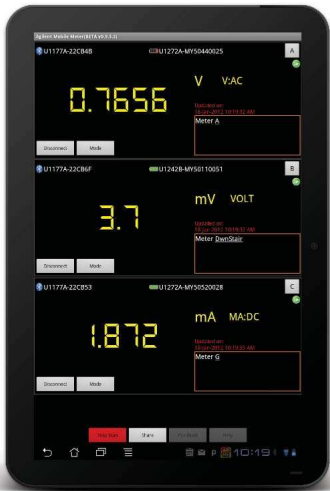
Figure 4. Up to three multimeters measurements with the Agilent Mobile Meter
