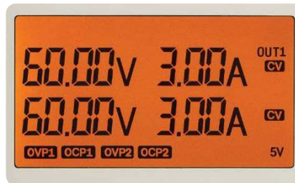
Figure 2. Backlight on/off feature with dual reading (voltage and current) on an LCD display
