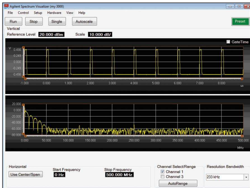
Figure 8: Measurement on pre-configured pulse waveform using the ASV and InfiniiVision X-Series oscilloscopes with WaveGen AWG
