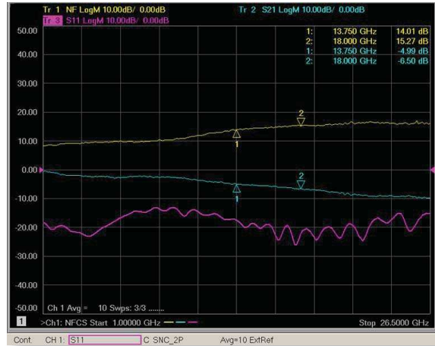
Figure 2. Typical link performance using the Agilent M9403A optical transmitter and M9404A optical receiver with the M9405A amplifier.
