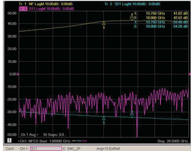
Figure 3. Typical link conversion loss using the Agilent M9403A optical transmitter and M9404A optical receiver without an amplifier.
