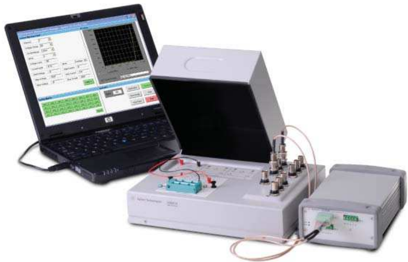
Figure 3. Sample setup of the U2941A connected directly to the U2722A source measure unit and fastened with the DIP socket module.
