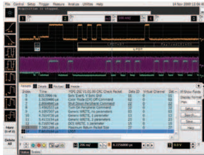
Trigger on and decode MIPI packets.
