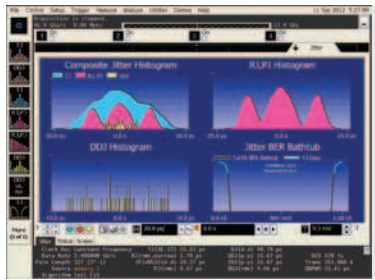
Analyze jitter plus RJ/DJ separation.
