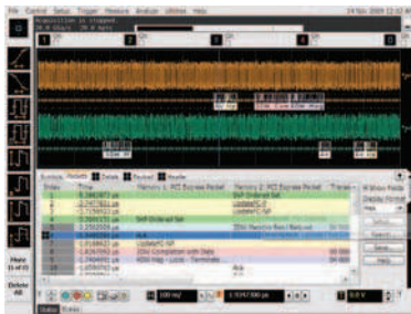
Trigger on and decode PCIe serial packets.
