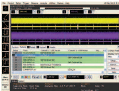
Isolate signal integrity problems from logic-level coding errors on bidirectional serial data streams.
