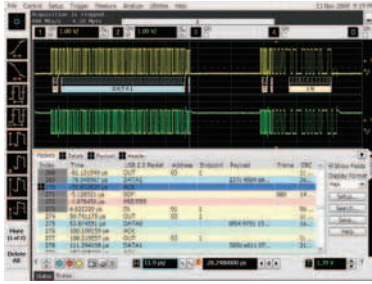
Trigger on and decode USB packets.
