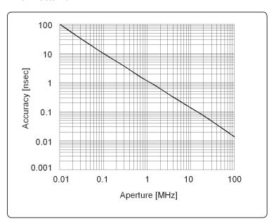
In general, the following formula can be used to determine the accuracy, in seconds, of specific group delay measurement:  $\pm$ phase accuracy (deg)/[360 x aperture (Hz)]
