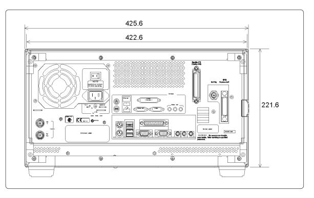
Figure 1-4. Dimensions (side view, in millimeters)
