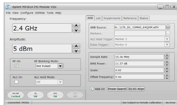
Figure 4. Agilent M9381A vector signal generator soft front panel.
