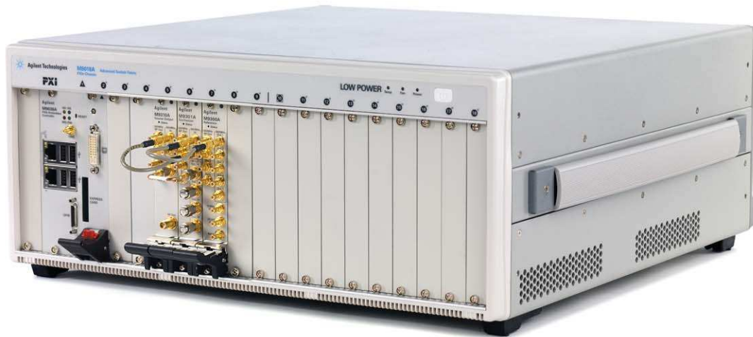
Figure 9. M9380A PXIe CW source with three modules consisting of the M9310A PXIe source output, M9301A PXIe synthesizer, M9300A PXIe frequency reference, an Agilent M9036A PXIe embedded controller all placed within the Agilent M9018A PXIe chassis.
