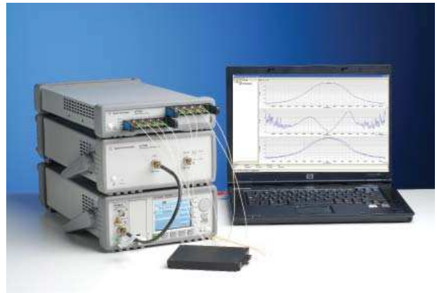
Figure 6. A very compact configuration for the IL/PDL Engine, to measure 8 channel devices in the C and L band
