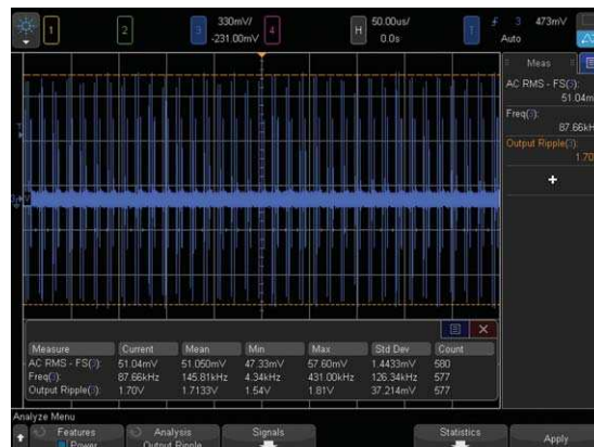
Figure 7 The output analysis includes characterizing the ripple component (either power line or switching) in output DC voltage.
