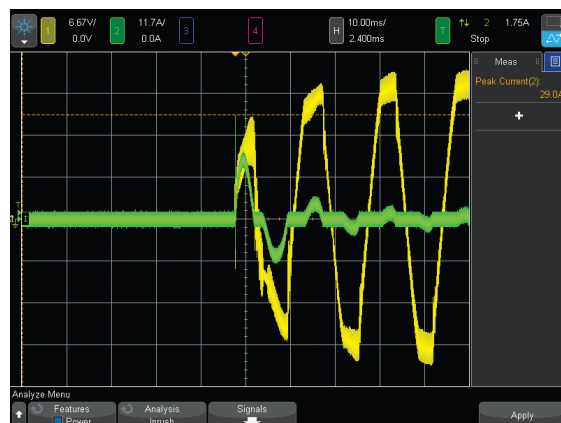
Figure 4 The Inrush current analysis measures the peak inrush current of the power supply when the power supply is first turned on.
