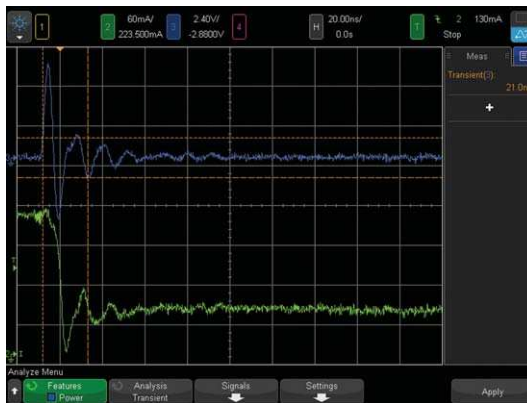
Figure 9 The transient analysis measures the load transient response of the DC output, namely the time taken for the DC output to stabilize during a load change.
