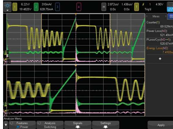
Figure 2. By measuring the switching loss and conduction loss, you can characterize the instantaneous power dissipation in a switching power supply.
