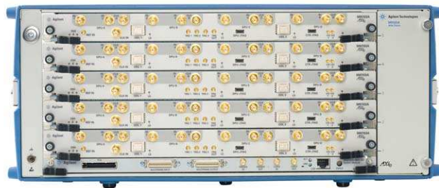
Figure 10. Five Agilent M9703A AXIe 12-bit digitizers installed in the Agilent M9505A 5-slot AXIe chassis to form a 40-channel 12-bit acquisition system.
