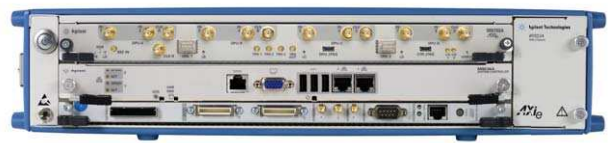
Figure 11. One Agilent M9703A AXIe 12-bit digitizers and one M9536A embedded AXIe controller installed in the Agilent M9502A 2-slot AXIe chassis.
