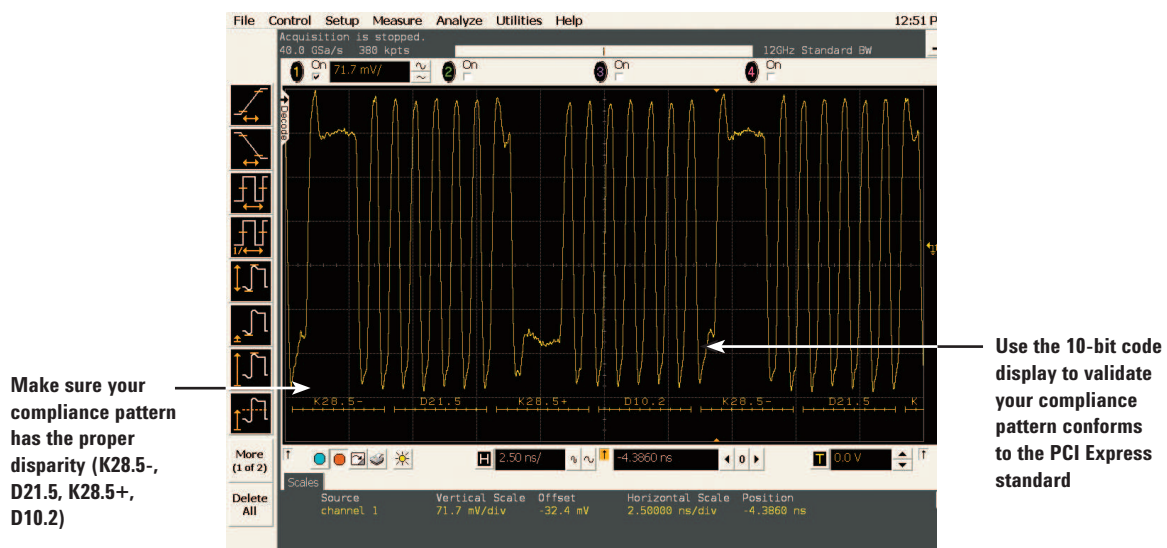
Figure 22. The 8b/10b decoded symbol information is shown below the appropriate portion of a PCI Express signal using the E2688A software.
