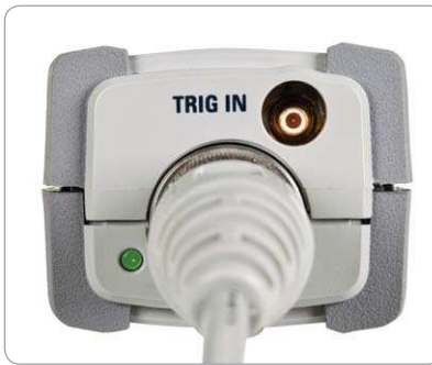
The external trigger input port on the U8481A.
