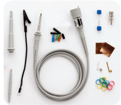
N2873A/N2894A passive probe with standard accessories
