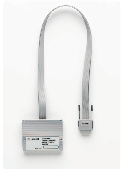
E5396A 16-channel soft touch connectorless probe
