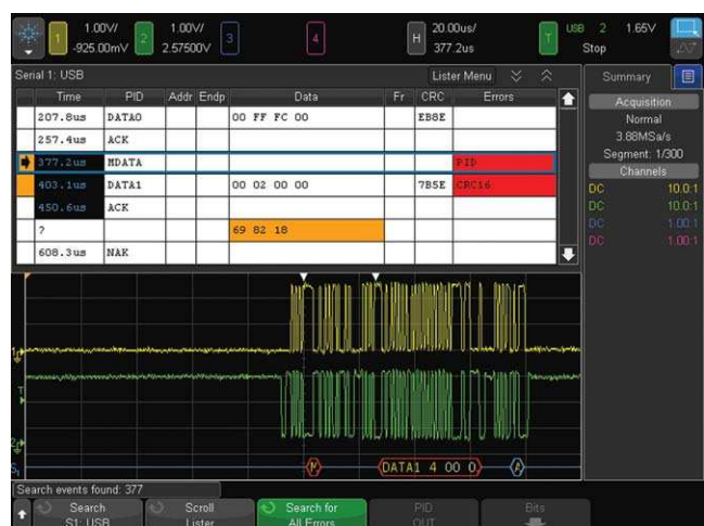
Figure 20: USB 2.0 trigger, decode and “lister” display.
