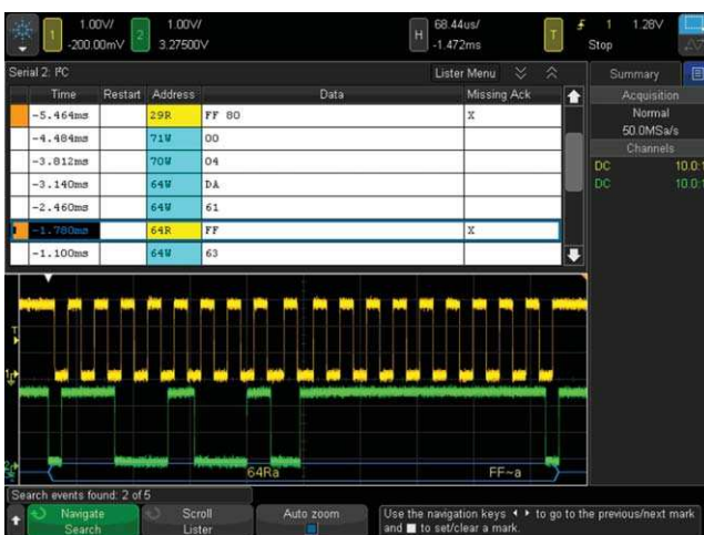
Figure 11: Using the error condition search, the 4000 X-Series quickly found 5 places with a missing acknowledgment in an I 2 C serial bus. The navigation feature moves between the errors and zooms automatically to show the error packet.
