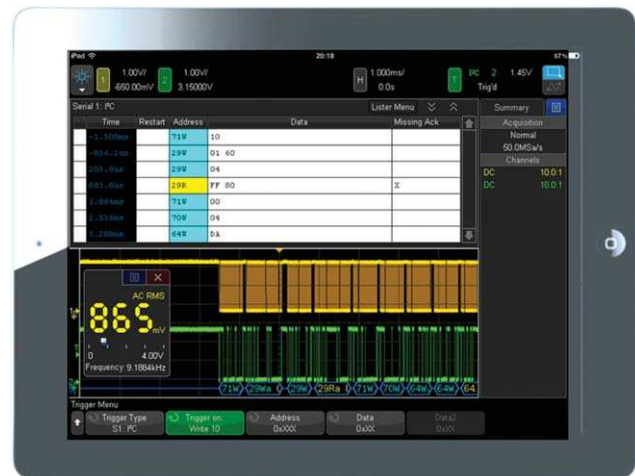
Figure 36: Tablet virtual front panel control.
