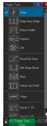
Figure 41: Wide array of advanced parametric trigger modes.
