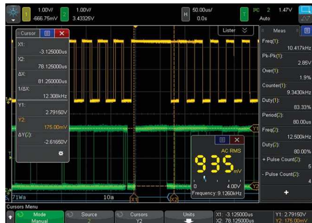
Figure 13: See 10 measurements, cursor information, and the DVM simultaneously by dragging the desired docking panel to any open area.
