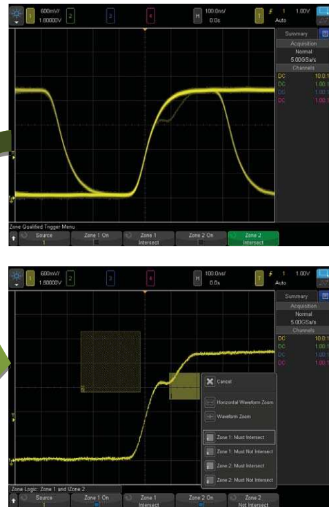
Figure 15. When you see anomalies, all you have to do is draw a zone box to trigger on them.
