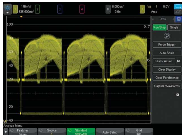
Figure 26: Triggering on 1080p HDTV signal analysis.
