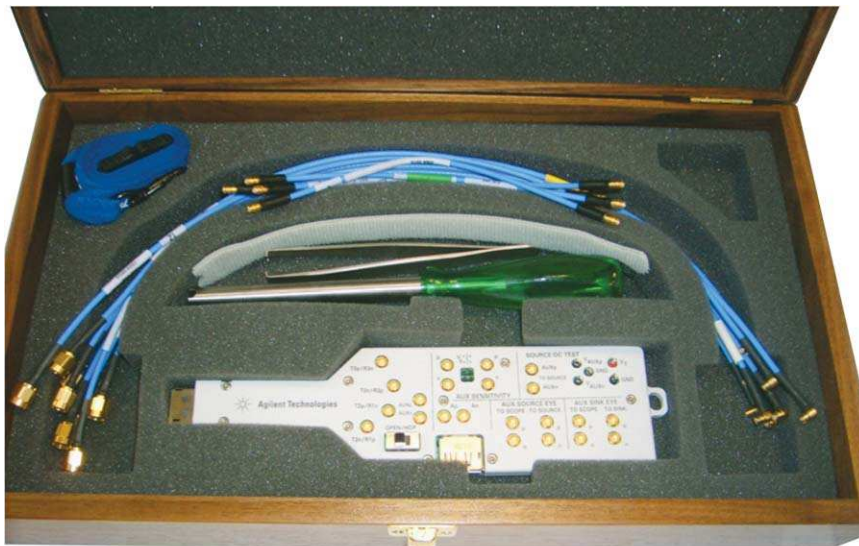
Figure 18. The Agilent W2641B DisplayPort test point adapter fixture
