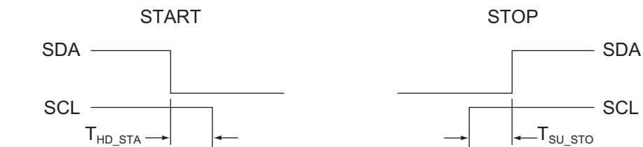
Figure 2: I²C Start and Stop Conditions;
