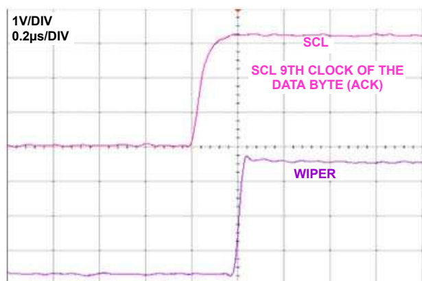
FIGURE 21. WIPER LARGE SIGNAL SETTLING TIME
