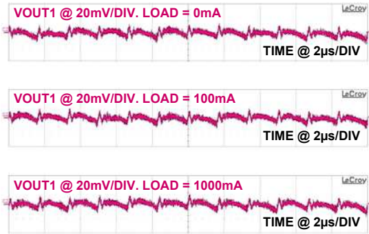
FIGURE 23. PWM1 OUTPUT RIPPLE, MODE = 5V (CCM)
